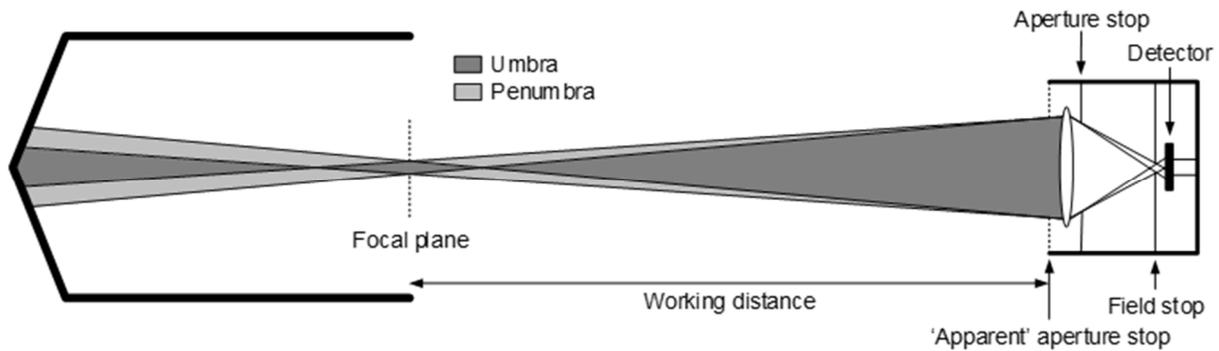
**Figure 1.** The field of view of a radiation thermometer is separated into an umbral region (dark shading) and a penumbral region (light shading). All the rays from the cavity surface within the umbral region that pass through the measurement spot at the focal plane are detected, but only some of those rays within the penumbral region are detected.
