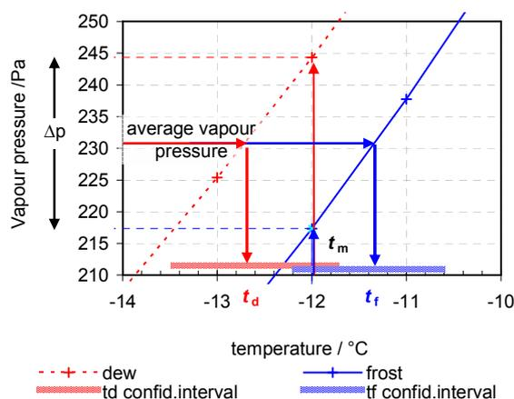
**Figure 7.** Determination of the corrected dew point or frost point and associated confidence intervals from the mirror temperature  $t_m$  when the condensate phase is unknown (see test for details).
