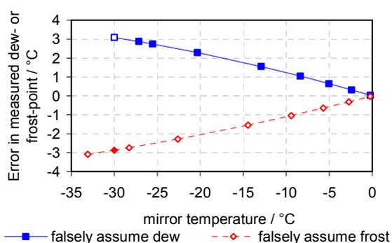
**Figure 6.** Error in dew point and frost point resulting from a false assumption of the phase of condensate on a chilled-mirror (see text for details).
