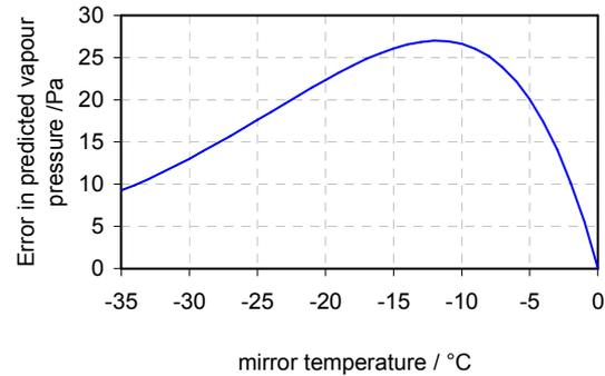
**Figure 4.** Maximum error in predicted vapour pressure for a false assumption of the condensate phase. This is just the difference  $\Delta p$  between the curves in Figures 1 to 3.
