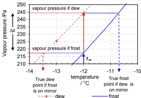
**Figure 3.** If the condensate phase is unknown, a range of vapour pressures is possible, depending on whether there is actually dew or frost, or both, on the mirror. Falsely assuming dew or frost leads to a maximum error of magnitude  $\Delta p$ .
