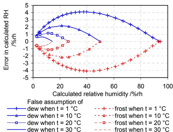
**Figure 9.** The error in calculated relative humidity based on a false assumption of dew or frost on a chilled mirror.
