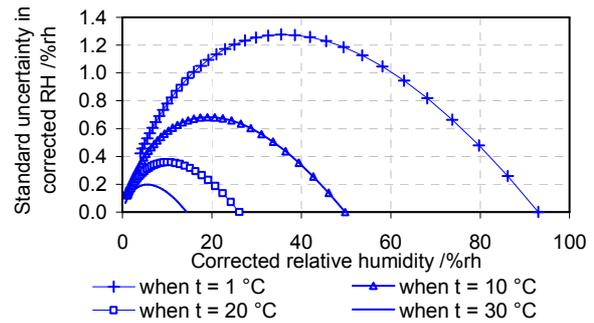
**Figure 10.** Standard uncertainty in corrected relative humidity calculated using the corrected dew point or frost point when the chilled-mirror condensate phase is unknown, for a range of dry-bulb temperatures.
