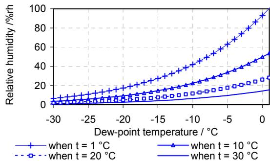
**Figure 8.** Relative humidity as a function of dry-bulb temperature  $t$ , for dew point temperatures less than  $0\text{ }^{\circ}\text{C}$ .
