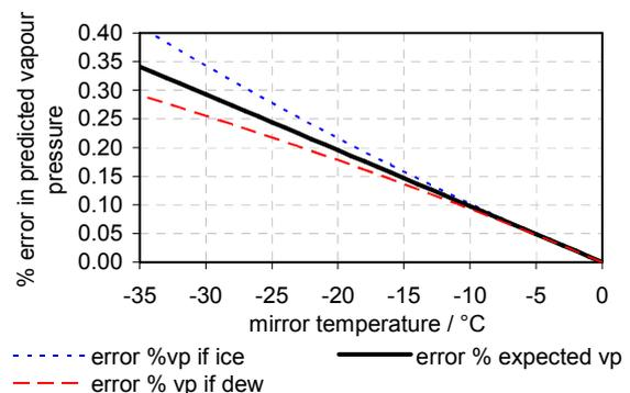
**Figure 5.** Error as a percentage of the actual vapour pressure if condensate is frost or dew (dotted and dashed lines) and error as a percentage of the "expected value" of vapour pressure (thick solid line, see text for details).
