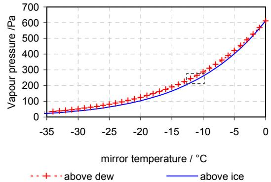
**Figure 1.** Vapour pressure above super-cooled dew and ice. Note that for the same vapour pressure, the super-cooled dew-point temperature is less than the frost-point temperature. The detail within the dashed-line box is shown in Figure 2.
