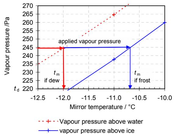
**Figure 2.** The same vapour pressure could result in a range of mirror temperatures  $t_m$  depending on whether there is super-cooled dew or frost on the mirror, or some transitional state as dew droplets freeze.
