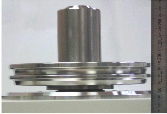
**Figure 2.** Measuring the fall rate of a gas-operated deadweight tester.
