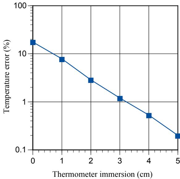
**Figure 3.** Plot of the thermometer error versus immersion. This should be a straight line on this semi-log graph (the vertical axis is logarithmic and the horizontal axis is linear).
