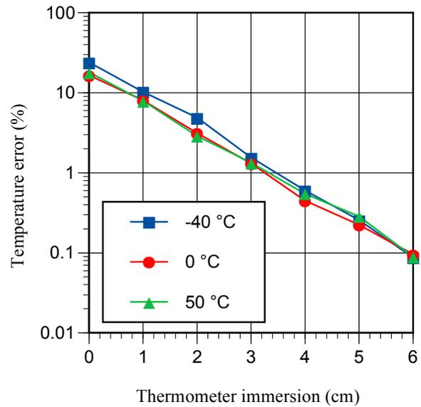
**Figure 4.** The temperature error graph should be similar at different temperatures. These results are for a dry-block calibrator.
