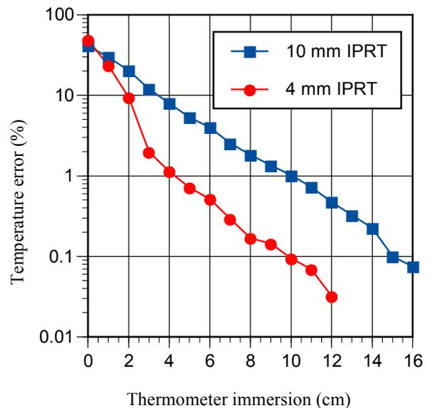
**Figure 5.** The immersion profile for two industrial platinum resistance thermometers in a calibration bath.
