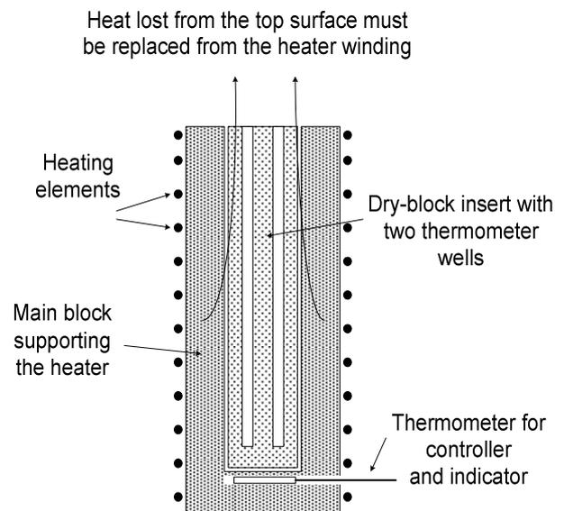
**Figure 2.** A typical dry-block calibrator. The heat flow from the heater to the top surface leads to a large temperature gradient in the block
