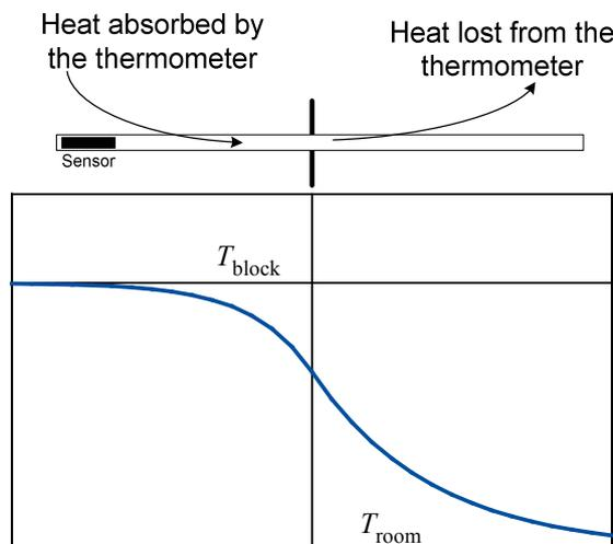
**Figure 1.** The typical temperature profile along the length of a thermometer.
