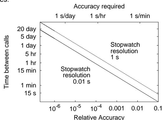
**Figure 2.** Graph showing the time required between calls to the talking clock versus the accuracy required from the calibration for the first and last uncertainties shown in Table 2.
