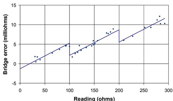
**Figure 2.** Typical error characteristic of an L&N 8078 resistance bridge. The points indicate measured errors and the 'sawtooth' shaped line indicates the calibration equation.
