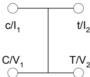
Figure 1. Connections for the 4-terminal shorting plug.
