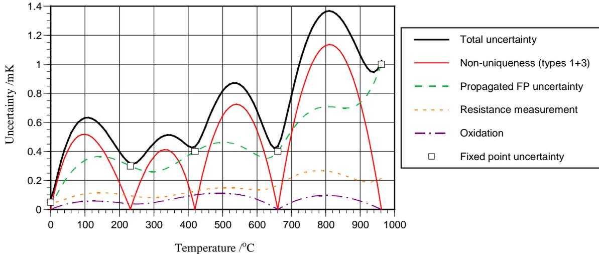
**Figure 9.5:** Contributions to total uncertainty for a long-stem SPRT calibrated over the water–silver subrange. It is assumed that the thermometer is to be used ‘in-house’. The calculated value includes the effects of non-uniqueness, the fixed-point uncertainties are as indicated, and the uncertainty in the resistance measurements is  $5 \mu\Omega$ . Contributions due to the uncertainty in use,  $u(R)$ , instability of the SPRT, and insulation breakdown have been omitted.
