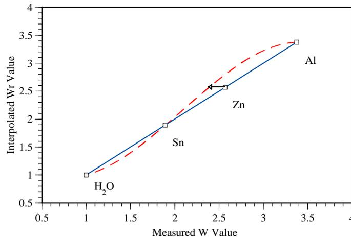
**Figure 9.1:** The influence of an error in a fixed-point measurement. The solid line shows an interpolation between the measured  $W$  values and the  $W_r$  values. The dotted line shows the effect of a small error in the measured  $W_{Zn}$  value. The difference in the two curves is the  $f_{Zn}(W)$  sensitivity coefficient for the water-aluminium subrange.
