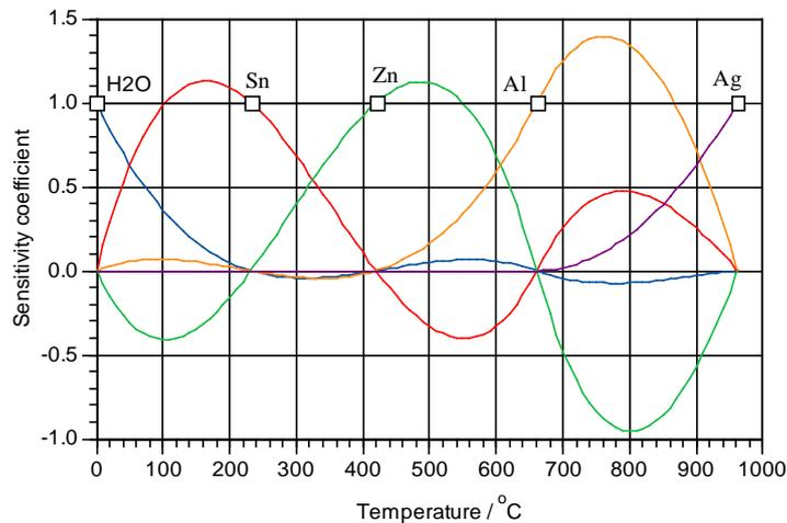
**Figure D.7:** The sensitivity coefficients for the water-silver subrange. The curves plot the propagated error in millikelvin for a 1 mK error at each of the fixed points. Below 660.323 °C (the aluminium point) the curves are identical to those in Figure D.6.
