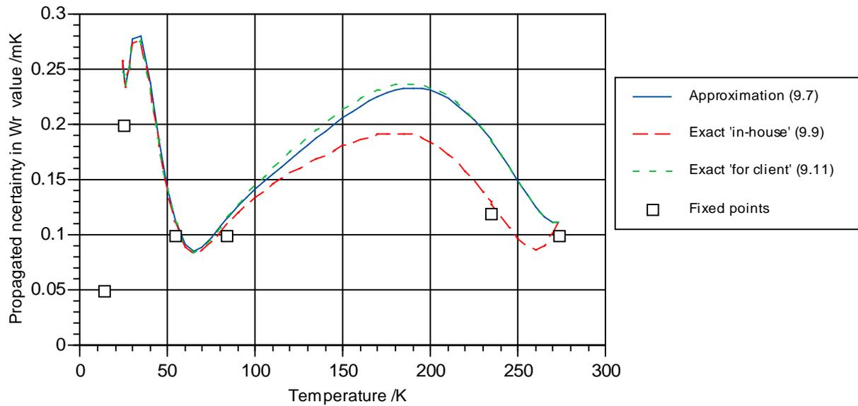
**Figure 9.2:** The propagated calibration uncertainty for the neon-water subrange, according to the different equations. The fixed-point uncertainties, as shown by the marked points, are indicative only. It is assumed that  $u(W)$ , the uncertainty in the  $W$  value in use, is zero.
