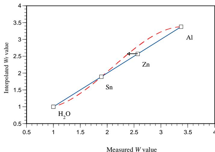
**Figure C.2:** The influence of an error in a fixed-point measurement. The solid line shows an interpolation between the measured  $W$  values and the  $W_r$  values. The dashed line shows the effect of a small error in the measured  $W_{Zn}$  value. The difference between the two curves is proportional to the  $f_{Zn}(W)$  function.
