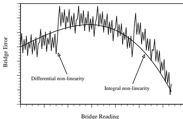
**Figure 8.2:** Graphical representation of the non-linearity of a resistance bridge including integral non-linearity (INL) and differential non-linearity (DNL). The smooth curve shows the INL only. The jagged curve is the sum of the INL and DNL.
