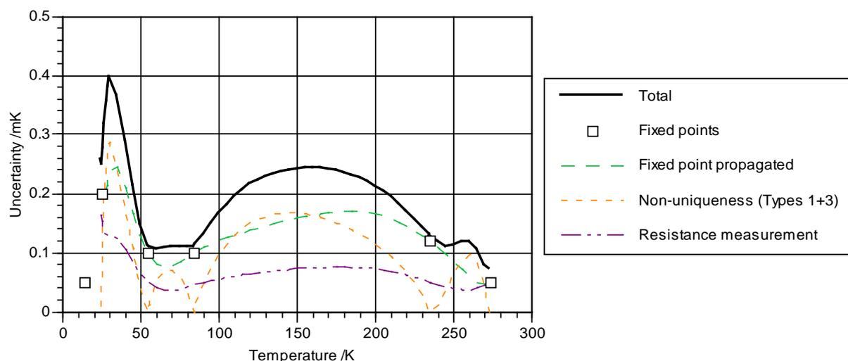
**Figure 9.4:** The contributions to the total calibration uncertainty for a 25  $\Omega$  capsule SPRT used ‘in-house’. The calculated value includes the effects of non-uniqueness, the fixed point uncertainties are as indicated, the uncertainty in the resistance measurements is 5  $\mu\Omega$ , and the in-use uncertainty  $u(R)$  is assumed to be zero.
