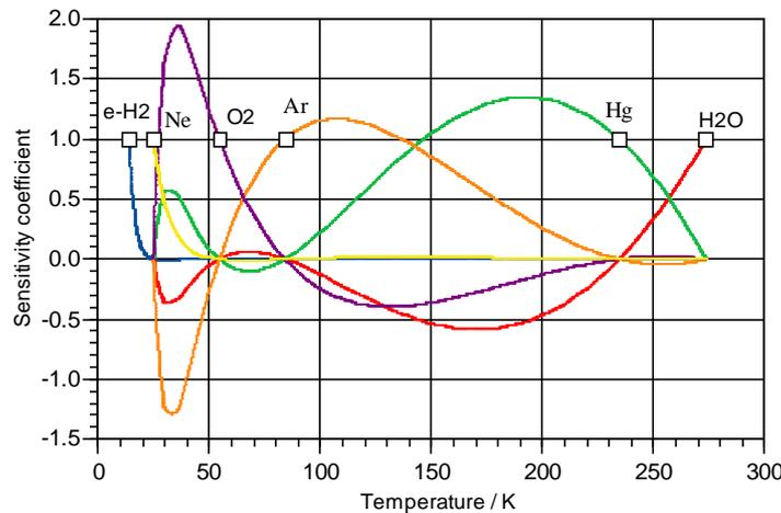
**Figure D.10:** The sensitivity coefficients for the neon-water subrange. The curves plot the propagated error in millikelvin for a 1 mK error at each of the fixed points. Note that the subrange extends only down to the Neon point (24.5561 K), although the hydrogen point is below this temperature.
