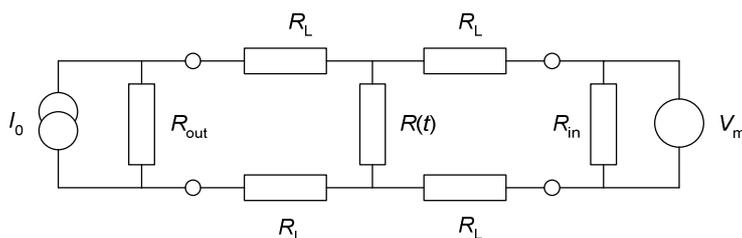
Figure 8.1: The equivalent circuit for a 4-terminal resistance measurement.
