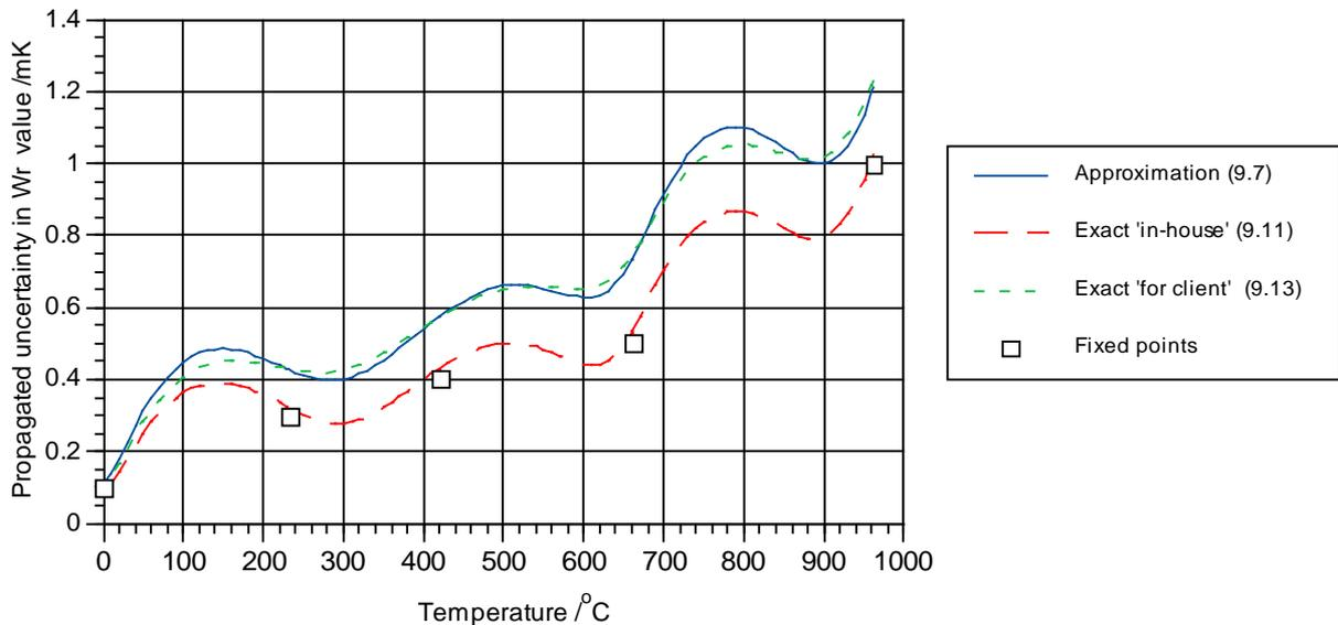
**Figure 9.3:** The propagated calibration uncertainty for the water-silver subrange, according to the different equations. The uncertainties for the fixed points, as shown by the marked points, are indicative only. It is assumed that  $u(W)$ , the uncertainty in the  $W$  value in use, is zero.
