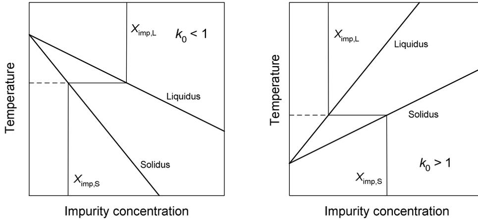
**Figure 2.2:** Simplified schematic representation of the binary phase diagrams for impurities at low concentrations. At temperatures above the liquidus, all of the material is liquid, below the solidus, all of the material is solid, and between the solidus and liquidus, solid and liquid coexist at equilibrium.
