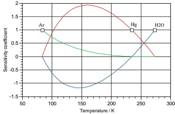
**Figure D.8:** The sensitivity coefficients for the argon-water subrange. The curves show the propagated error in millikelvin for a 1 mK error at each of the fixed points.
