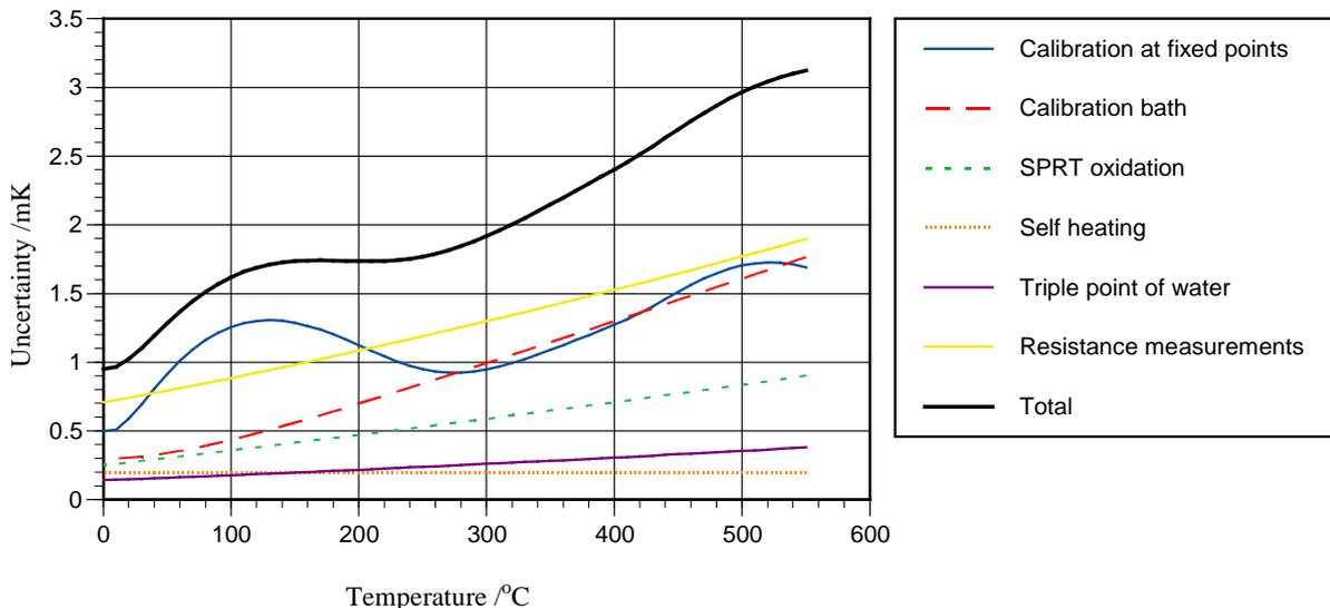
**Figure 9.6:** A numerical example for the total uncertainty for an SPRT used in a calibration bath.
