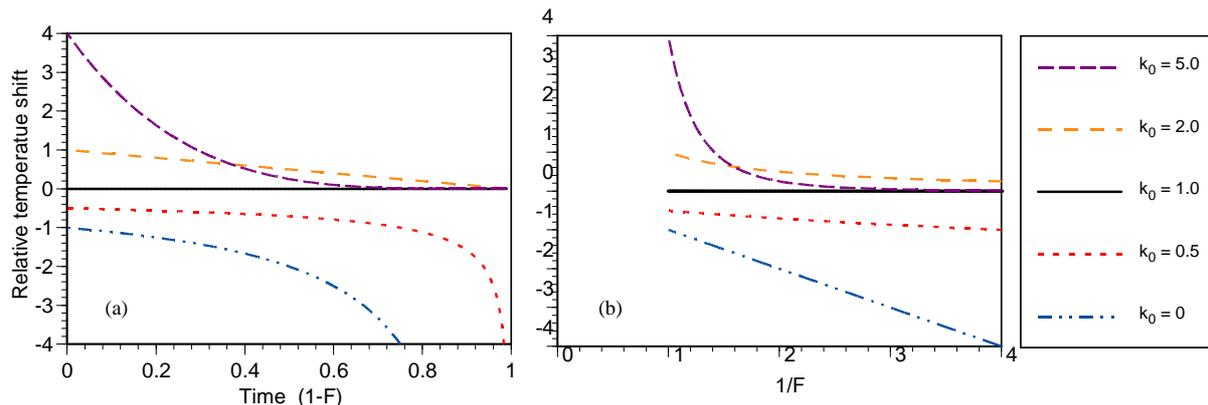
**Figure 2.3:** Idealised freezing curves for fixed points with impurities with different distribution coefficients according to the factor  $(k_0 - 1)F^{k_0 - 1}$  of Equation (2.16): (a) plotted against the frozen fraction  $1 - F$  (approximately proportional to elapsed time), (b) plotted against  $1/F$  (linear in the case for  $k_0 = 0$ ).
