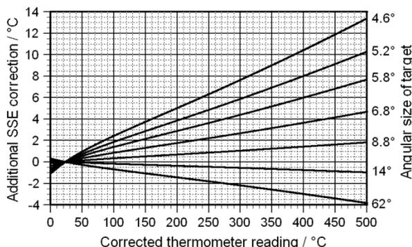
**Figure 8.** Alternative method for graphing the additional SSE corrections, as a function of temperature for a number of different angular target sizes. The points plotted in Figure 7 corresponds to points somewhere on this graph. The additional corrections for a target size of  $11.4^\circ$  are zero for all temperatures.
