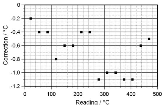
**Figure 5.** Corrections determined during the comparison phase of a calibration using a blackbody with an angular size of  $11.4^\circ$ . The correction is equal to the expected reading minus the actual reading.
