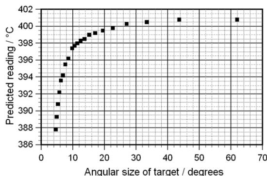
**Figure 6.** Predicted readings for the same conditions as in Figures 3 and 4, but for the blackbody at  $400^\circ\text{C}$ . The points have been calculated using equation (3) from the measurements plotted in Figure 4.
