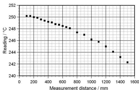
**Figure 3.** A set of readings as a function of measurement distance for a blackbody at  $T = 249.7\text{ }^\circ\text{C}$ , with aperture diameter of  $d = 120\text{ mm}$  and effective emissivity of  $\epsilon_{\text{bb}} = 0.9910$ . The ambient temperature was  $T_{\text{amb}} = 23\text{ }^\circ\text{C}$ .
