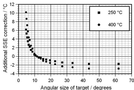
**Figure 7.** Corrections required to account for the SSE in addition to those found during the comparison phase of the calibration, for blackbody temperatures of  $250^\circ\text{C}$  and  $400^\circ\text{C}$ . These are the differences between the readings for an angular target size of  $11.4^\circ$  (which was the blackbody size during the comparison phase) in Figures 4 and 6, respectively, and the corresponding readings for the particular target size along the x-axis.
