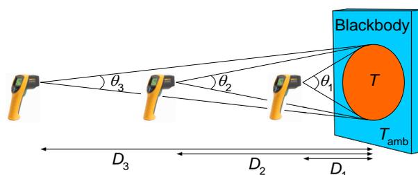
**Figure 2.** Characterising the SSE by measuring the same blackbody, at temperature  $T$ , over different distances  $D_1, D_2, D_3, \dots$ . Each measurement corresponds to a different angular target size  $\theta_1, \theta_2, \theta_3, \dots$ . The ambient temperature is  $T_{\text{amb}}$ .
