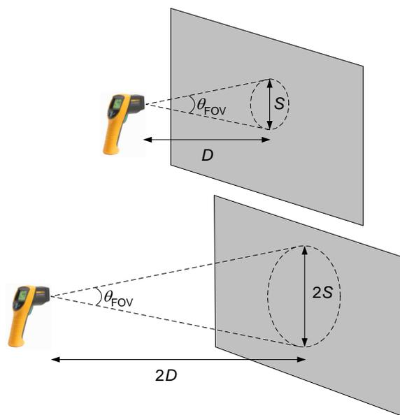
**Figure 1.** Ideally, doubling the measurement distance,  $D$ , doubles the spot size,  $S$ , of the nominal field of view, keeping the angular field of view,  $D:S$  or  $\theta_{FOV}$ , constant.
